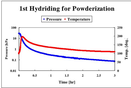
Fig. 3. Change of hydrogen pressure and temperature during hydriding for powderization at room temperature.
