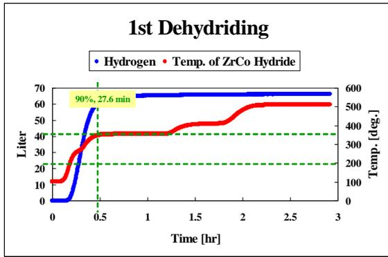
Fig. 4. Change of amount of hydrogen pressure and temperature during dehydriding.
