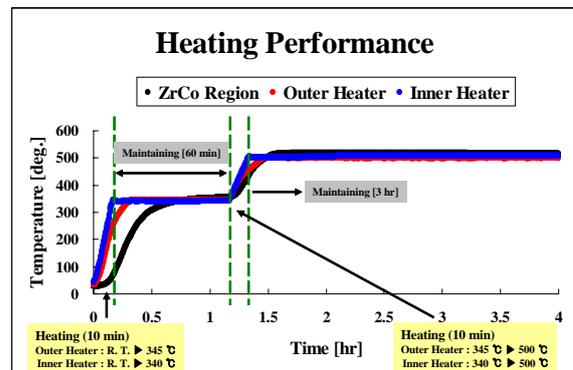
Fig. 2. History of the ZrCo region temperature according to the operating inner/outer heater
