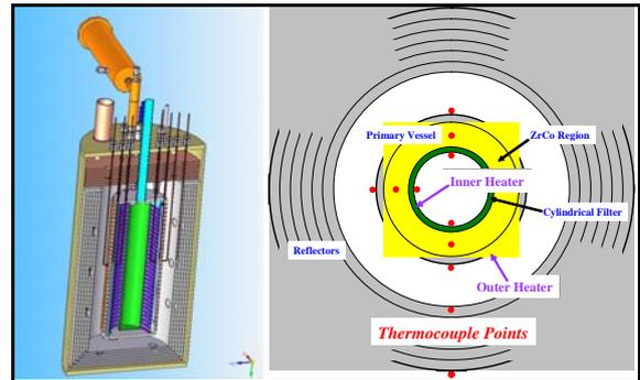
Fig. 1. Vertical Cross-section view of the ZrCo bed and thermocouple points
