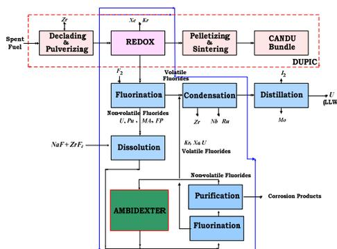
Fig. 1. AMBIDEXTER-DUPIC Fuel Cycle Flow Diagram
