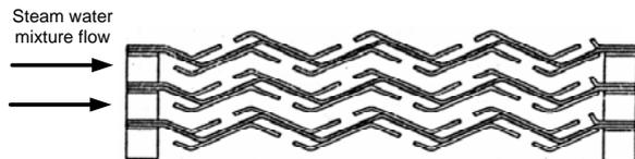
Figure 1 Flow channel of the steam dryer
