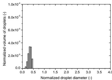
Figure 4 Normalized volume of moisture after the dryer vane
