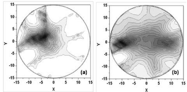
Fig. 2. Images taken by the industrial SPECT when only one cylinder is filled with radioactive tracer (a), and both cylinders are filled with radioactive tracer (b).
