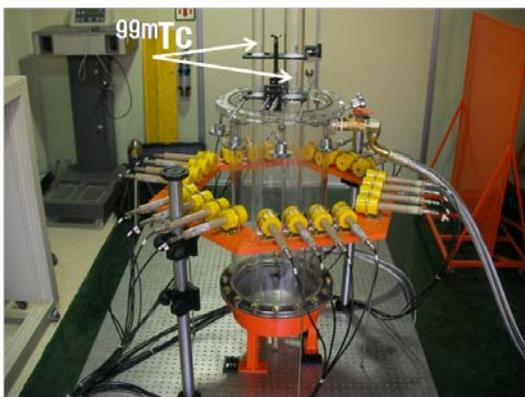
Fig. 1. Experiment set-up with the industrial SPECT developed at KAERI. There are two cylindrical sources containing <sup>99m</sup>Tc inside the cylindrical basin.
