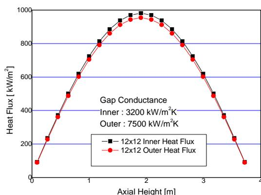
Fig. 3 Axial heat flux variations for inner and outer surfaces of the hottest annular fuel
