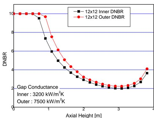
Fig. 4 DNBR variations along the axial direction for inner and outer channels at the hottest annular fuel
