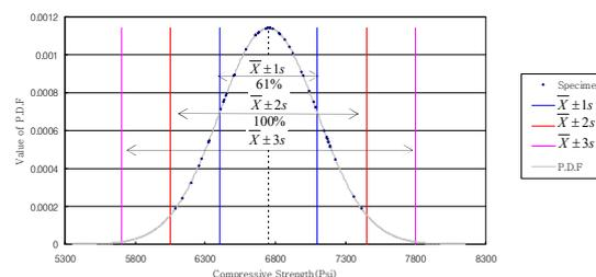
Fig. 2 Normal Frequency Distribution Curve of Compressive Strength in SWN Unit 1&2
