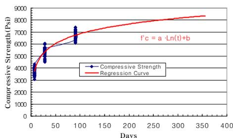
Fig. 1 Compressive Strength of Concretes
