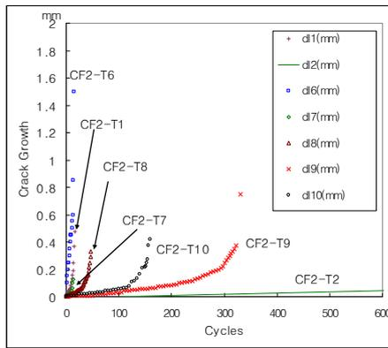
Fig. 3 Crack length growth of the 2mm defect specimens
