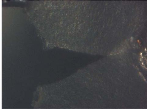
Fig.6 Instable crack growth at 161 cycles for CF2-T10 (x120)
