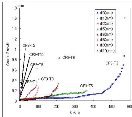
Fig. 4 Crack length growth of the 3mm defect specimens
