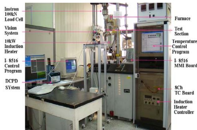
Fig. 1 A creep-fatigue crack test facility
