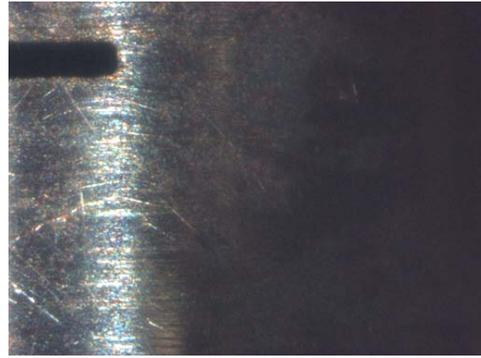
Fig.5 Defect area at the start of the test for CF2-T10 (x120)
