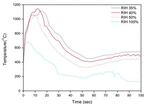
Figure 2 Fuel sheath temperature for RIH break LOCA
