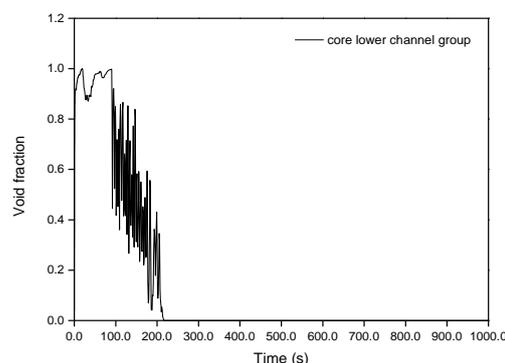
Figure 5 Integrated channel void in core lower channel
