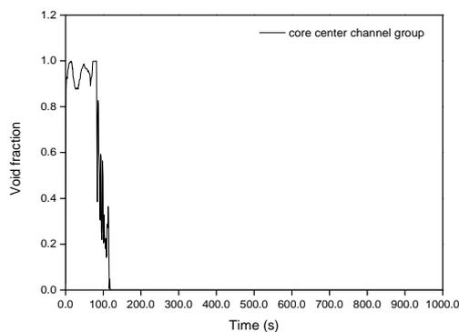
Figure 4 Integrated channel void in core center channel
