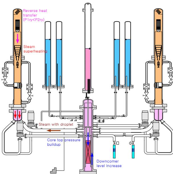
Figure 1 Schematic diagram of the steam binding phenomenon in the ATLAS
