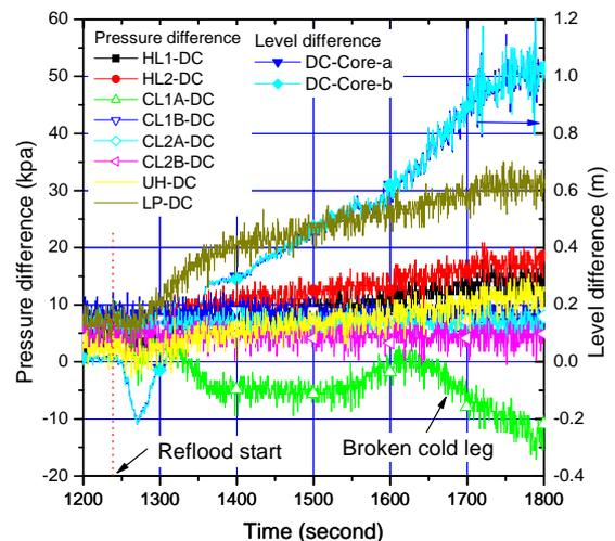
Figure 2 Behavior of pressure difference relative to downcomer and core-downcomer level difference
