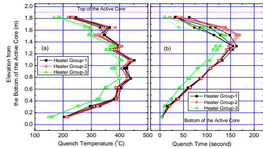
Figure 4 Behavior of quench temperatures and quench times along the axial elevation of the active core
