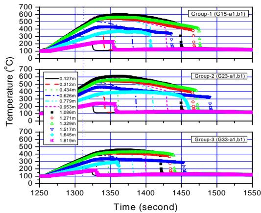
Figure 3 Axial surface temperature distributions of three core heater rods during LB-CL-14 (Group-1, 2 & 3)
