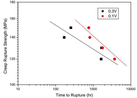
Fig. 4. Creep rupture strength of FM steels at 650°
