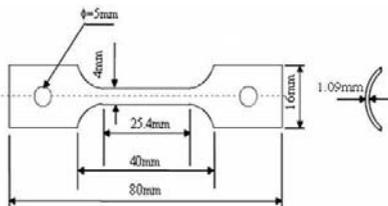
Figure 1. Shape and dimensions of the slow strain rate tensile specimen.
