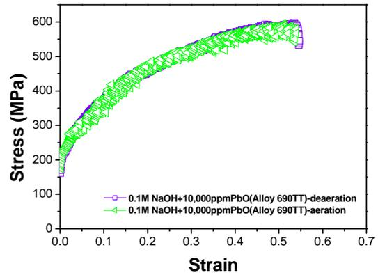
Figure 2. Stress-strain curves of Alloy 690 TT in 0.1M NaOH + 10,000ppm PbO with/without deaeration at 315°C.
