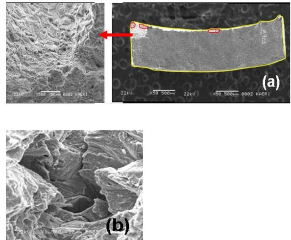
Figure 3. SEM micrograph of the fracture surface(a) and specimen surface morphologies(b) Alloy 690 TT in 0.1M NaOH+10,000ppm PbO without deaeration at 315°C.
