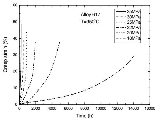
Fig. 1. Creep curves obtained with the elapsed times for different stress levels at 950°C for Alloy 617.
