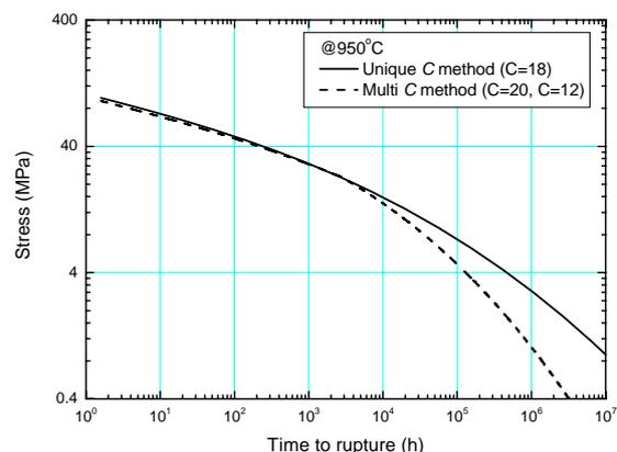
Fig. 4. Comparison of predicted creep strength for the unique  $C$  and multi  $C$  methods at  $950^\circ\text{C}$ .
