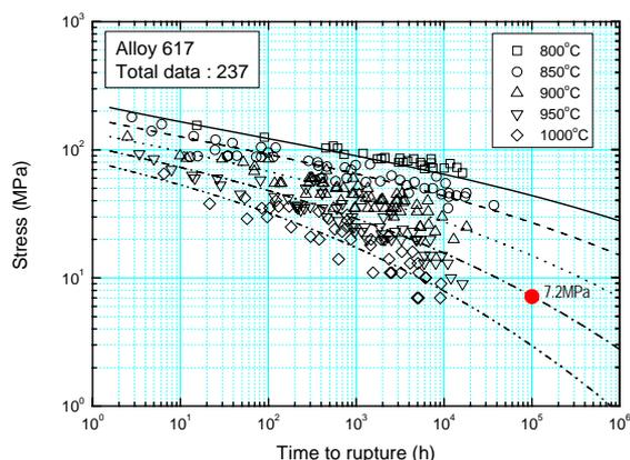
Fig. 3. Creep strength predicted by a unique value of  $C = 18$  at temperatures of 800 to  $1000^\circ\text{C}$  of Alloy 617.
