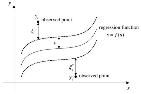
Fig.1. The parameters for the support vector regression.
