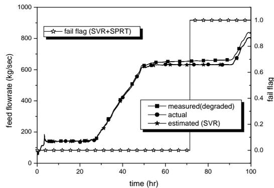
Fig. 3. Monitoring of the feedwater flow rate in cases of artificial degradation
