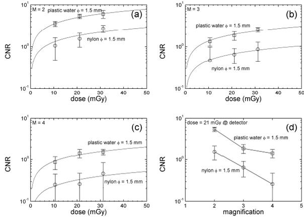
Fig. 3. Calculated CNRs for the contrast phantom with respect to dose and magnification.
