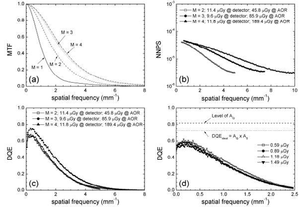
Fig. 1. Fourier analyses of the imaging performances of the detector with respect to magnification. (a) MTF, (b) Normalized NPS, and (c) DQE. (d) DQE with respect to dose at the entrance surface of the detector without magnification (or  $M = 1$ ).
