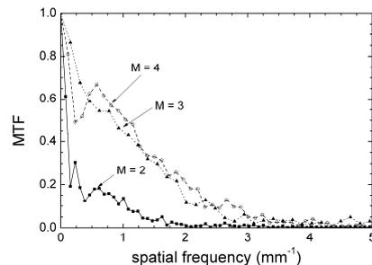
Fig. 2. MTF in CT images with respect to  $M$ . MTF results were estimated based on Hankel transform of transaxial images reconstructed from the wire phantom.
