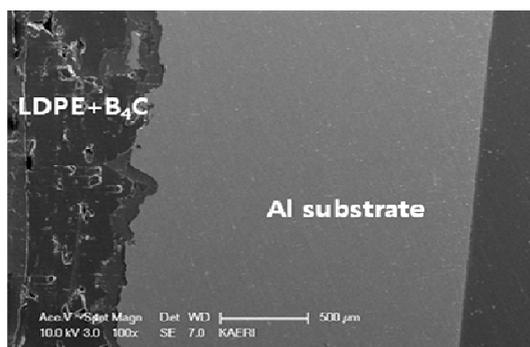
Fig. 3. Cross-sectional SEM image of LDPE-20wt.%  $B_4C$  composite powder coating on Al substrate.
