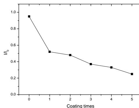
Fig. 4. Change in thermal neutron absorbing efficiency of LDPE- $B_4C$  composite powder coating on Al substrate with respect to the coating times.
