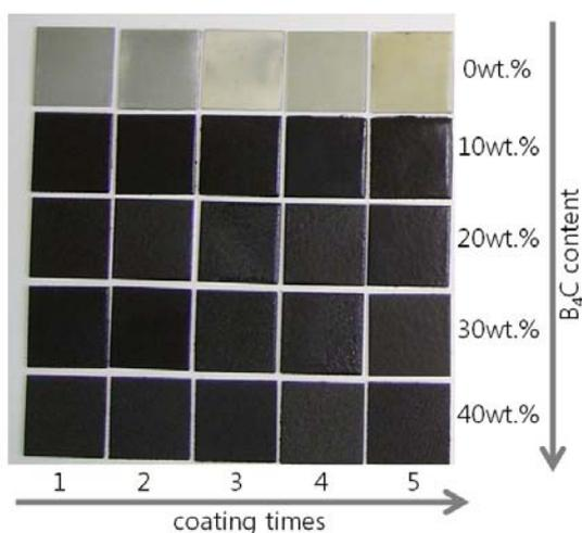
Fig. 2. Optical micrographs of LDPE- $B_4C$  composite powder coating on Al substrate with different  $B_4C$  contents and coating times by the help of flame spraying method.
