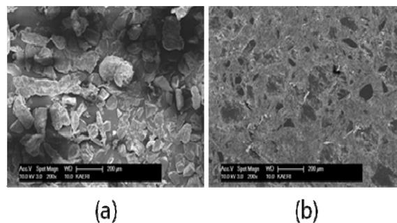
Fig. 1. SEM micrographs of (a) surface and (b) cross-section of 20wt.% B<sub>4</sub>C containing LDPE composite powder.
