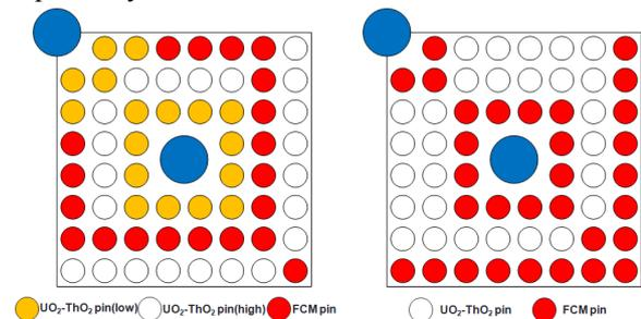
Fig. 1 Configuration of the new fuel assembly (1/4)
