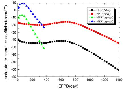
Fig. 5 Comparison of MTC for the new core and typical LWR core
