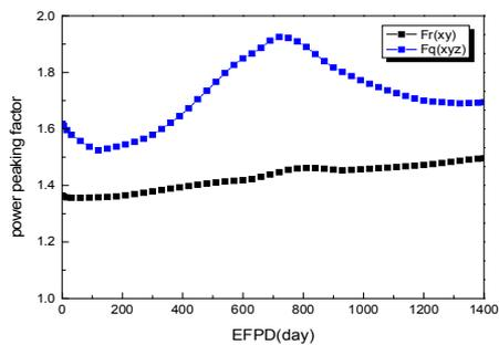
Fig. 4 power peaking factor for the new core
