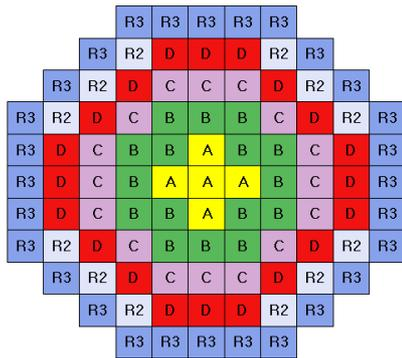
Fig. 2 Radial configuration of the new core
