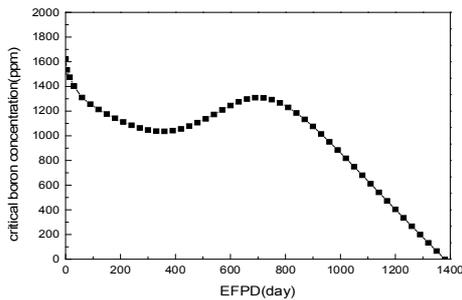
Fig. 3 Critical boron concentration for the new core
