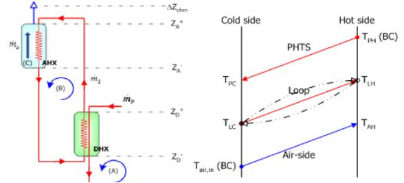
Fig. 1. DHRS heat removal paths (left) and temperature distribution concept (right).
