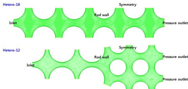
Fig.1. CFD model on FCM 12by12 and FCM 16 by 16 with conventional 16 by 16 assembly
