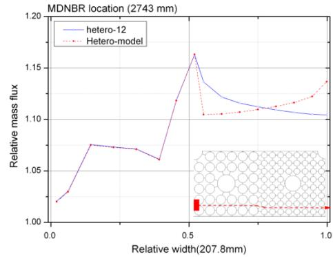
Fig.4. Axial flow distribution on Hetero-12 case
