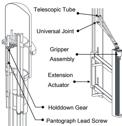
Fig. 3 Pantograph mechanism and gripper assembly in PGSFR
