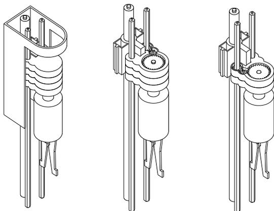
Fig. 4 Driving mechanism of the PGSFR gripper assembly
