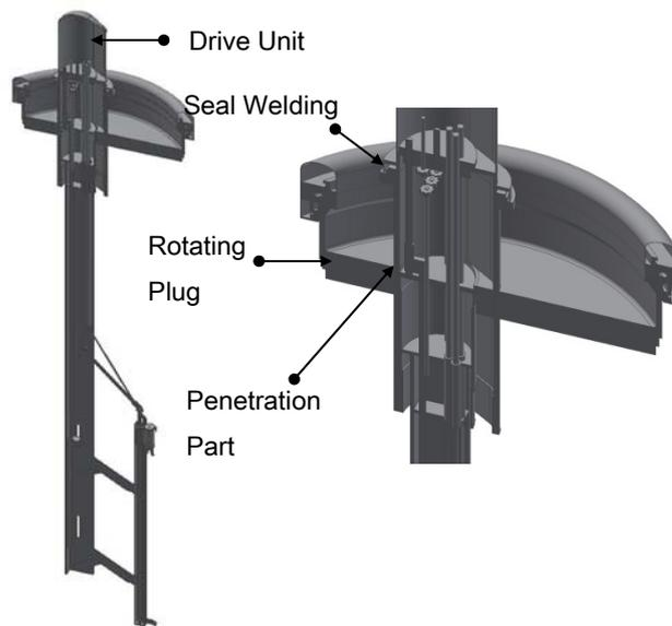
Fig. 6 IVTM penetration and seal welding part in PGSFR
