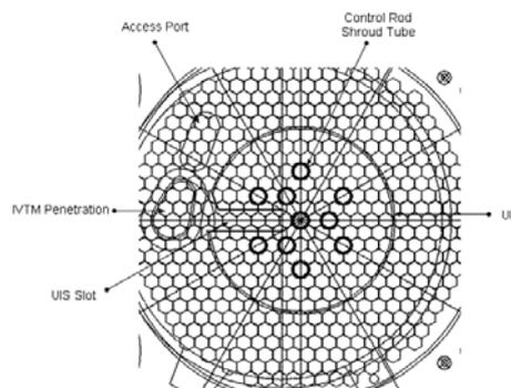
Fig. 5 Top view for the IVTM and upper internal structure in PGSFR
