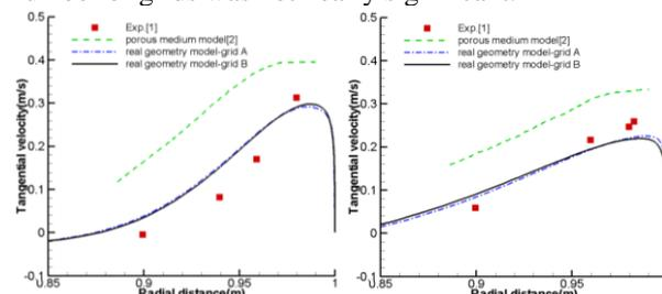
Fig. 3. Tangential velocity profile at 30 degree (left) and 60 degree (right) from the horizontal centerline in the counter-clockwise direction
