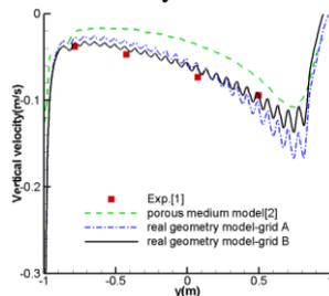
Fig. 2. Vertical velocity profile at the vertical centerline (x=0)
