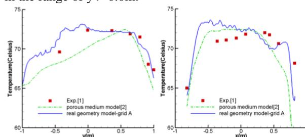
Fig. 4. Temperature profile at the vertical centerline (x=0; left) and the horizontal line (y=0.57m; right)
