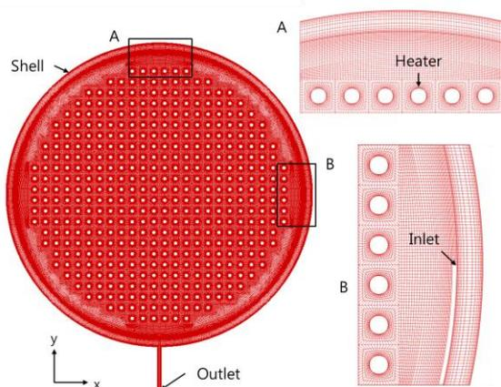
Fig. 1. Computational domain and grid system
