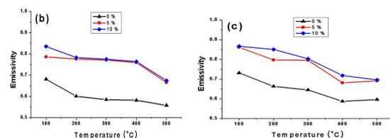
**Fig. 2** Oxidation effects and temperature dependencies of TE for IG-110 (b) and PCEA (c).
