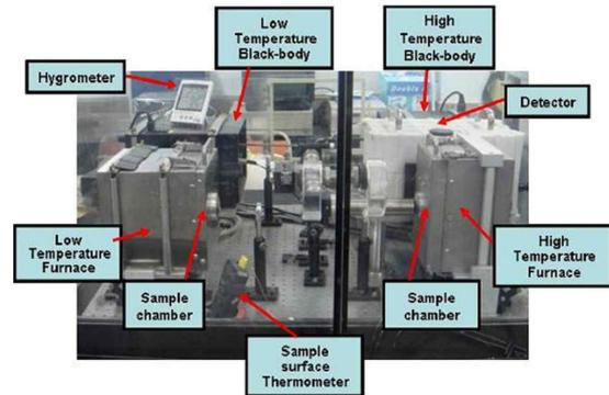
**Fig. 1** Infra-red spectrum measurement system (FT-IR, MIDAC M2400-C, 4000-400  $\text{cm}^{-1}$ , Resolution: 0.5  $\text{cm}^{-1}$ , 5-20 $\mu\text{m}$ , 100-500°C).
