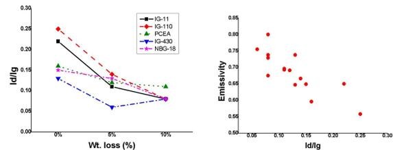
**Fig. 3** Raman results (Id/Ig - Weight Loss) and Emissivity-Id/Ig relationship for 5 grades examined.
