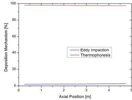
Fig. 3. Deposition mechanisms along the test pipe.
