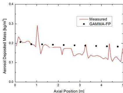
Fig. 2. Aerosol deposition along the test pipe.
