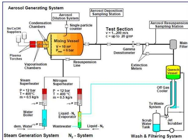
Fig. 1. The STORM experimental facility.
