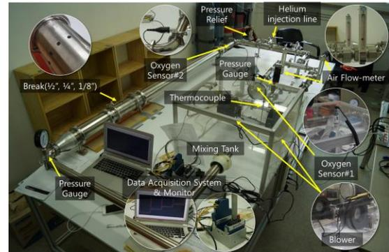
Figure 2. Small Break Air-Ingress Experimental Facility.
