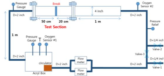
Figure 1. Schematic of Small Break Air-Ingress Experimental Facility.
