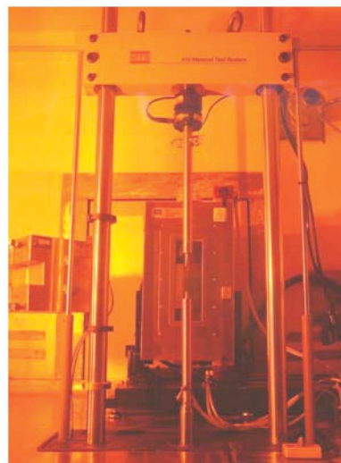
Fig. 3. Equipment System Used to Measure Mechanical Properties in a Hot Cell
