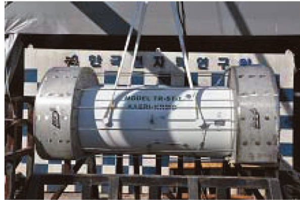
Fig. 2.7. Deformation of the Cask after the Side Drop Test
