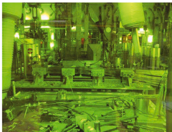
Fig. 6. FFTF Fuel Assembly Being Disassembled in HFEF.
