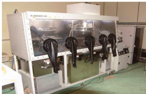
Fig. 5. High-throughput Electrorefiner Equipped with Graphite Cathodes
