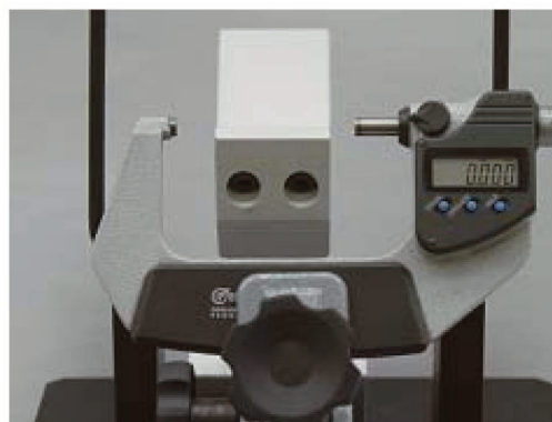
Fig. 4. Micrometer Used to Measure Irradiation Growth
