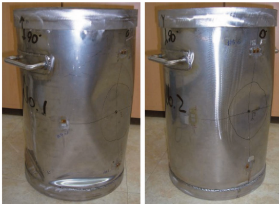
Fig. 2.3. Comparison of Deformations between the Sequential Drop Test and Puncture-only Test
