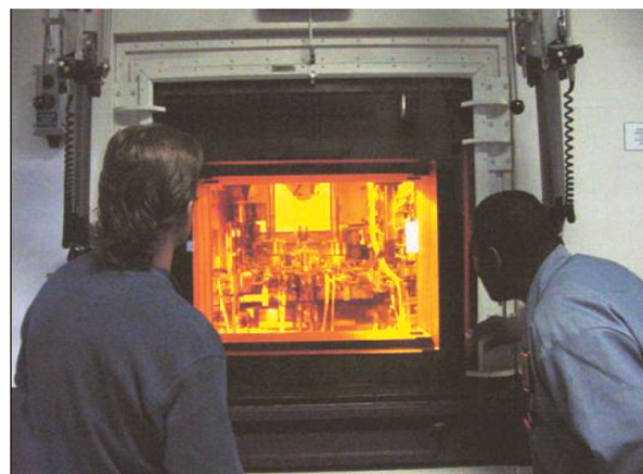
Fig. 7. Electrorefiner Viewed through Hot Cell Window in FCF Argon Cell.
