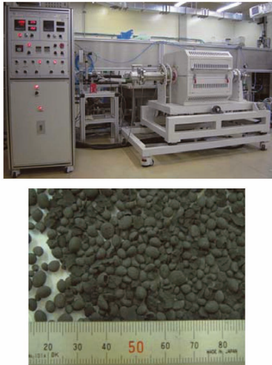
Fig. 2. A Rotary Voloxidizer (Left) and \text{UO}_{2+x} Granules (Right)
