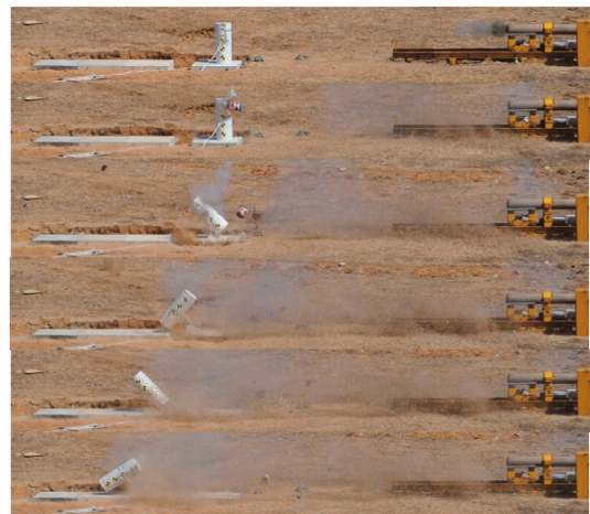
Fig. 3.6. Cask Behavior after Impact
