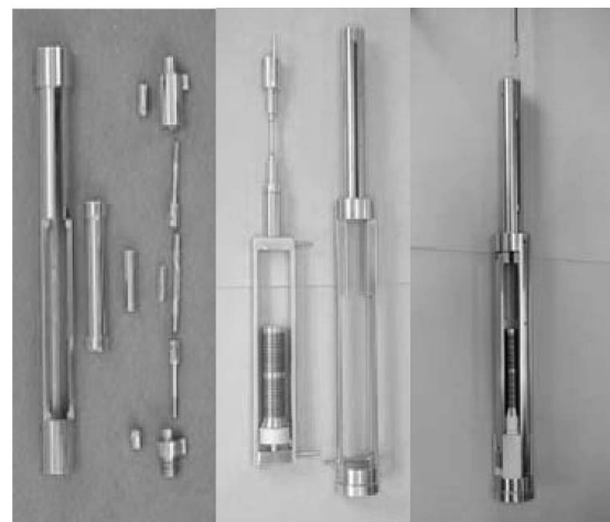
Fig. 4. Capsule for a Creep Test
