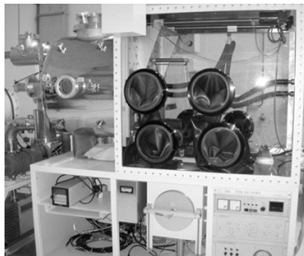
Fig. 10. The Lab-scale U Ingot Casting Equipment
