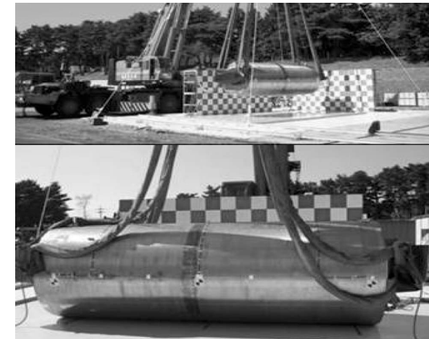
Fig. 7. Horizontal Drop Test of Canister
