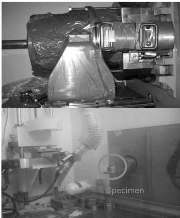
Fig. 2. Specimen Cask Fitted with the Adaptor on a Hot Cell Wall (Upper) and a Specimen Basket of Cask Inside a Hot Cell (Lower)
