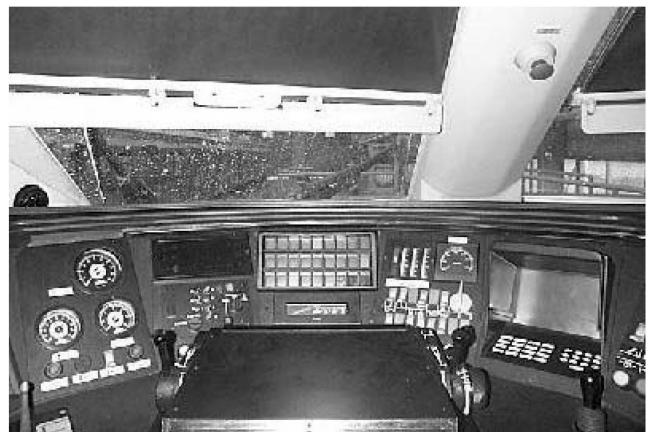
Fig. 6. The Cab of KTX – Its Layout
