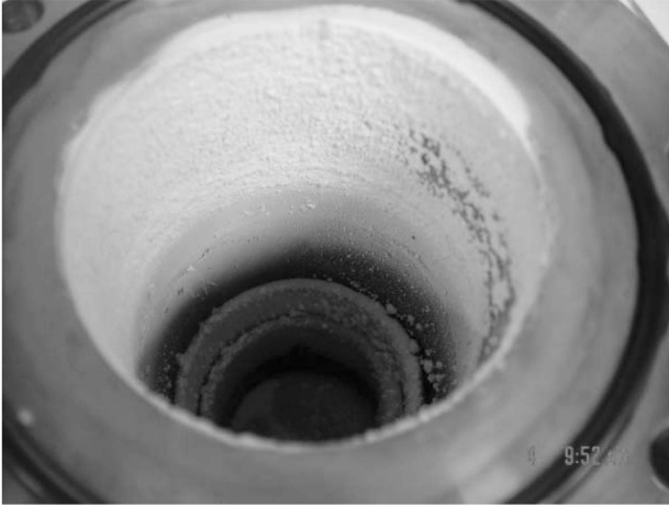
Fig. 1. Inside of an Electrolytic Reducer Covered with Vaporized Salts after Electrolytic Reduction
