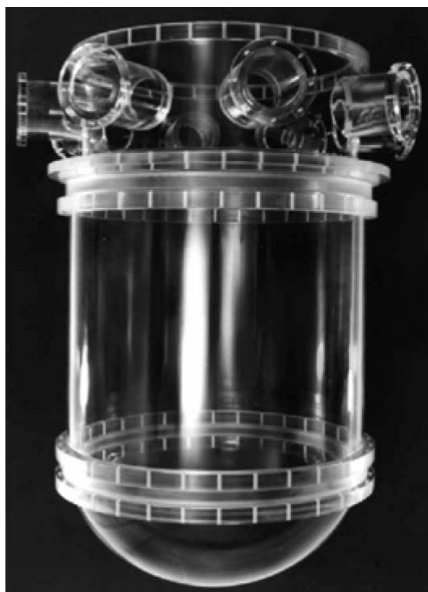
Fig. 1. Reactor Model of the ROCOM Test Facility
