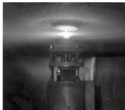
Fig. 1. (a) A Schematic Illustration and (b) a Photograph of the Centrifugal Atomization Process
