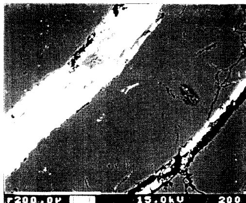
Fig. 11. Backscattered Electron Image of Quartzite. Layers of Uranium Containing Mineral are Shown as Light Tone
