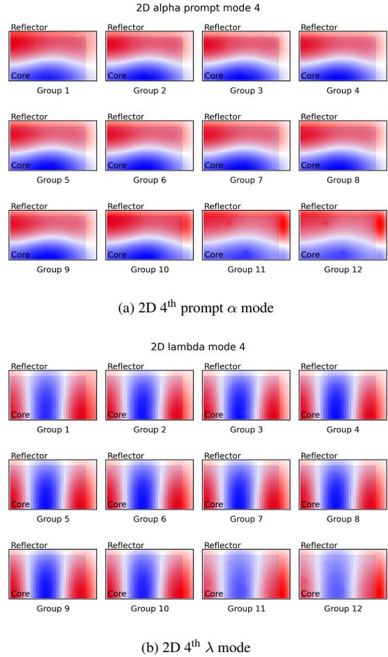
Figure 2: The 4<sup>th</sup> prompt  $\alpha$ -mode as returned by ARPACK and the corresponding  $\lambda$ -mode in 2D geometry.
