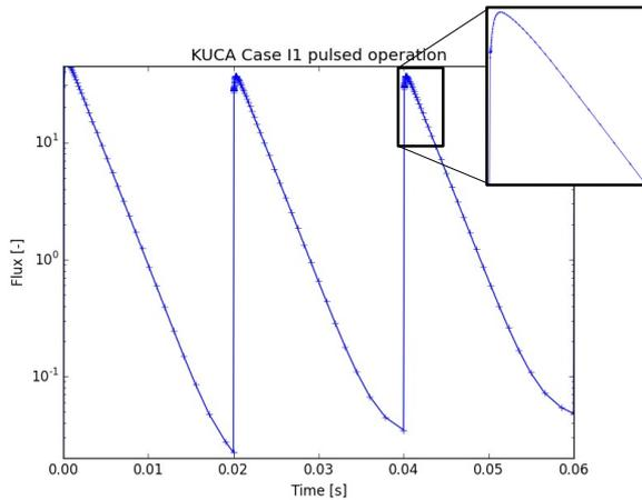
Figure 3: Simulation of pulsed neutron experiment in KUCA (benchmark case I-1).
