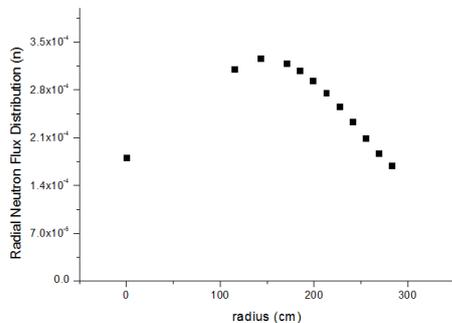
Fig.5. Relative value of radial neutron flux distribution
