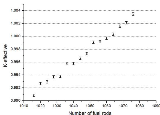
Fig.5. Loading Curve of k-effective
