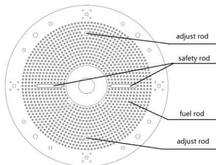
Fig.2. Grid plate front view
