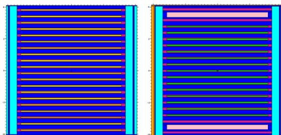
(a)standard fuel assembly (b)control fuel assembly
