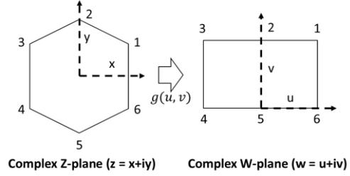
Fig. 2. Conformal mapping of a hexagon to a rectangle
