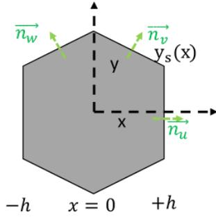
Fig. 1. A hexagonal node and its coordinate system
