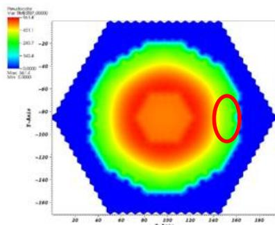
Fig. 4. Model core power distribution and removed control rod position (circle).
