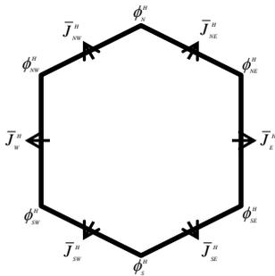
Fig. 1. Boundary conditions for hexagonal geometry.
