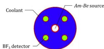
Fig. 1. Top view of the boron meter.
