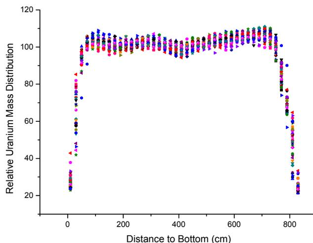
Fig. 1. Relative Axial Uranium Mass Distribution from fuel rod samples.
