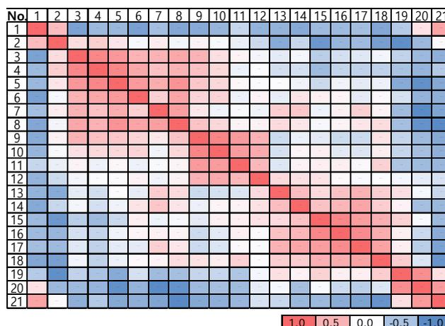
Fig. 2. Correlation Coefficients Matrix for Axial Uranium Mass Distribution
