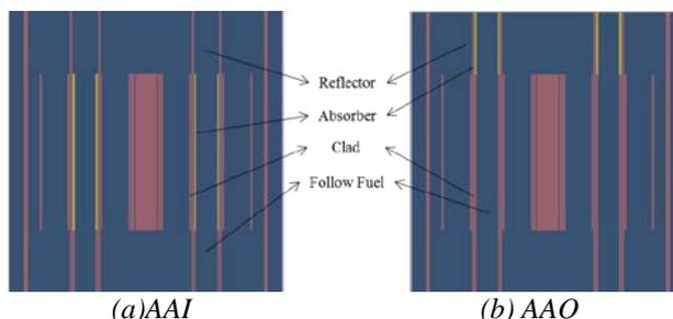
Fig. 3. Axial cut of the JRR-3M reactor whole-core model.
