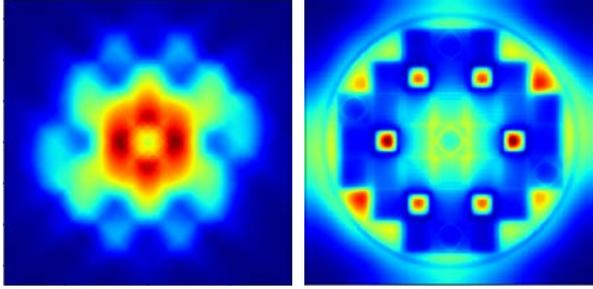
Fig. 4. Flux distribution results of on the 1st and 7th energy group for the 2D whole-core AAI case
