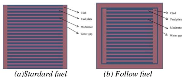
Fig. 1. Standard fuel and follow fuel assembly model with SHARK
