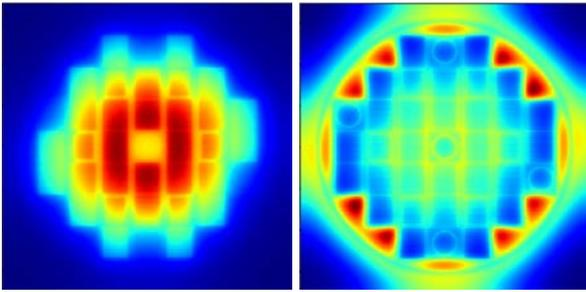
Fig. 5. Flux distribution results of on the 1st and 7th energy group for the 2D whole-core AAO case
