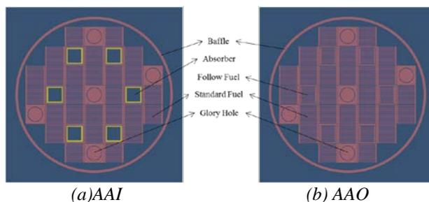
Fig. 2. Radial cut of the JRR-3M reactor whole-core model.
