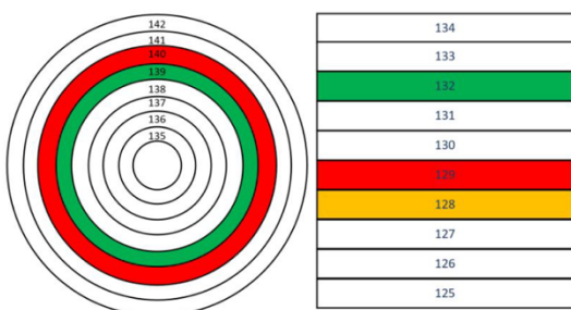
Fig. 13. Layered depiction of the maximum neutron flux positions within the reactor core at 100 seconds
