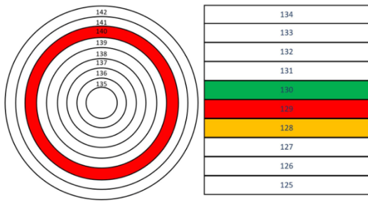
Fig. 12. Maximum neutron flux positions within the reactor core at 50 seconds
