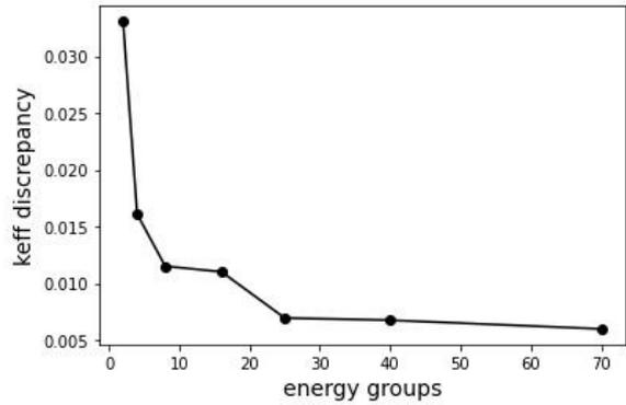
Fig. 3. keff discrepancy for different group structures
