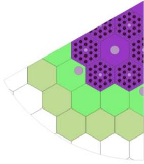
Fig. 4. A sixteenth of whole core with assembly height
