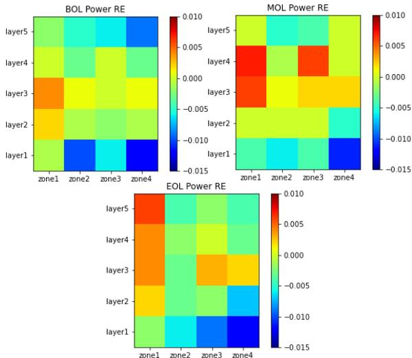
Fig. 6. The relative errors of power distribution at typical burnup points for Case 2
