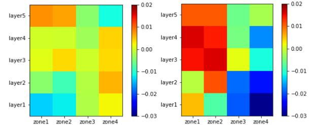
Fig. 5. Power relative error for WCM and SCM homogenization model
