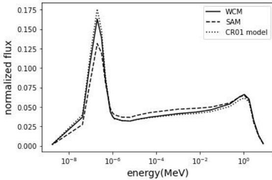
Fig. 4. Energy spectrum for Zone 1 fuel block in different models
