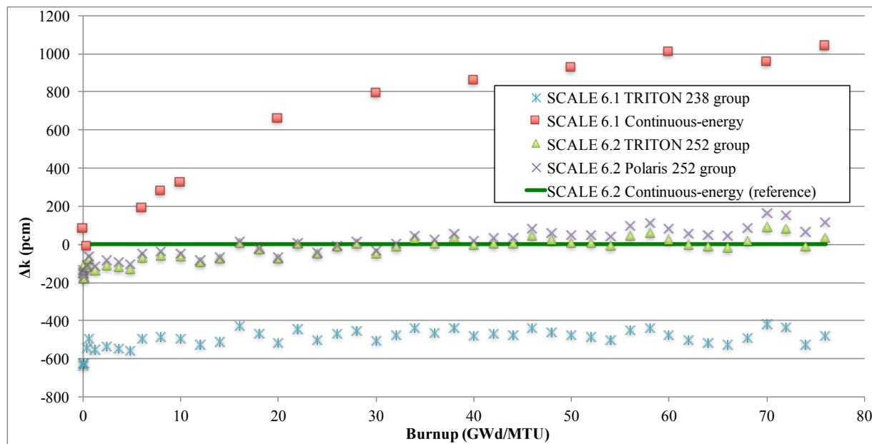
Fig. 7. Comparison of computational biases as a function of burnup.
