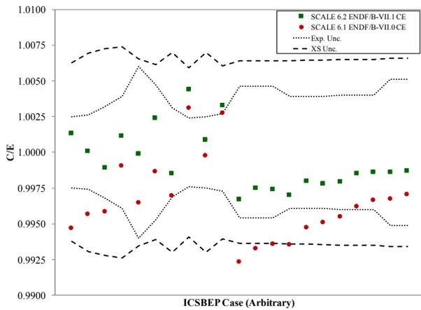
Fig. 1. SCALE C/E results for International Criticality Safety Benchmark Evaluation Project thermal mixed oxide critical systems.
