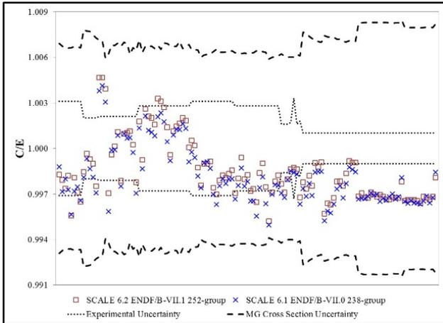
Fig. 3. Comparison of SCALE 6.1 and SCALE 6.2 MG results for 123 LCT benchmarks.
