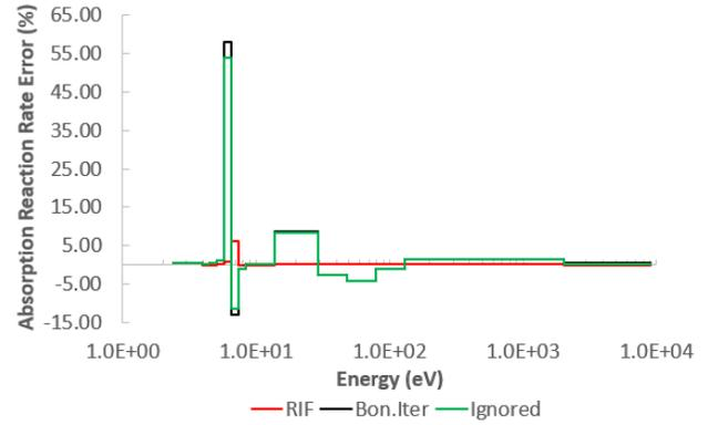
Fig. 9. U-235 Absorption Reaction Rate Error for 1.0 w/o MOX fuel.
