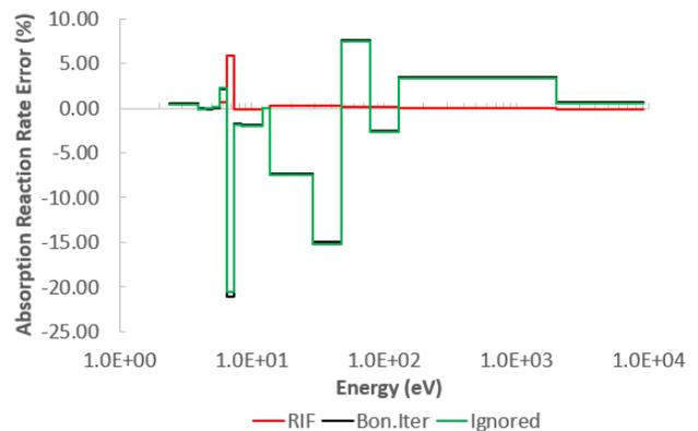
Fig. 11. Pu-239 Absorption Reaction Rate Error for 1.0 w/o MOX fuel.
