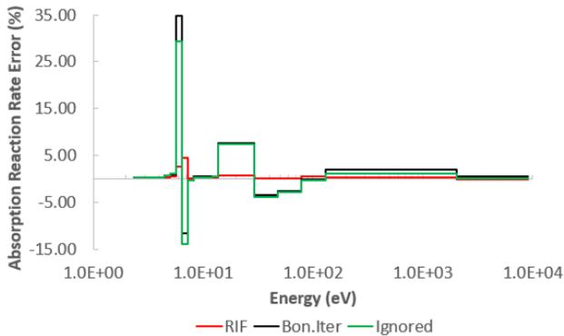
Fig. 5. U-235 Absorption Reaction Rate Error for 5.0 w/o UO<sub>2</sub> fuel.
