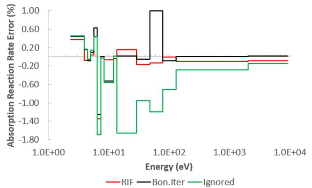
Fig. 10. U-238 Absorption Reaction Rate Error for 1.0 w/o MOX fuel.
