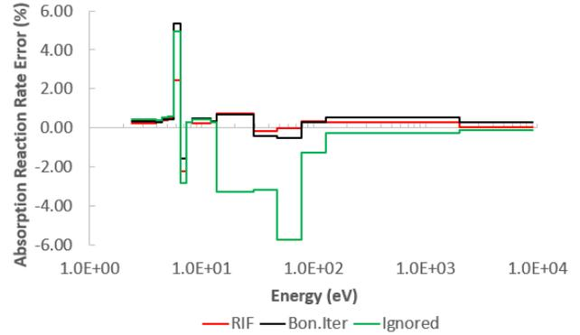
Fig. 6. U-238 Absorption Reaction Rate Error for 5.0 w/o UO<sub>2</sub> fuel.
