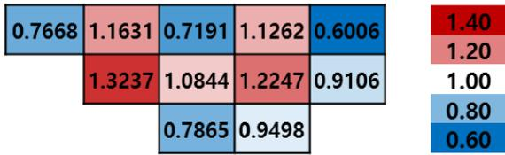
Fig. 14. Reference assembly normalized power distribution of the rodded core
