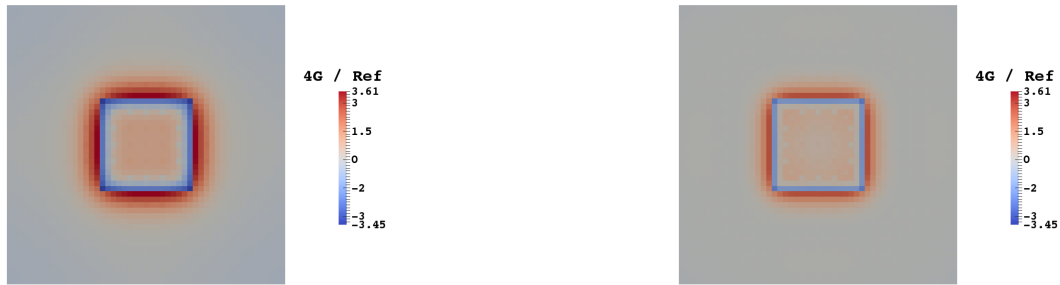
Fig. 1: Pin power comparisons between the 4-group SP_3 with P_3 (left) and TP_3 (right) and the best-estimate calculations.
