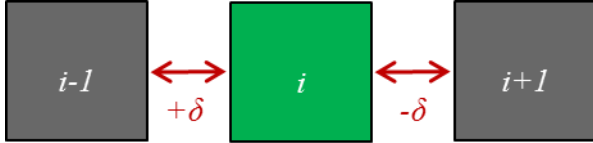
Fig 1. Preservation of delta gap sizes on both sides of a vibrating fuel assembly i .
