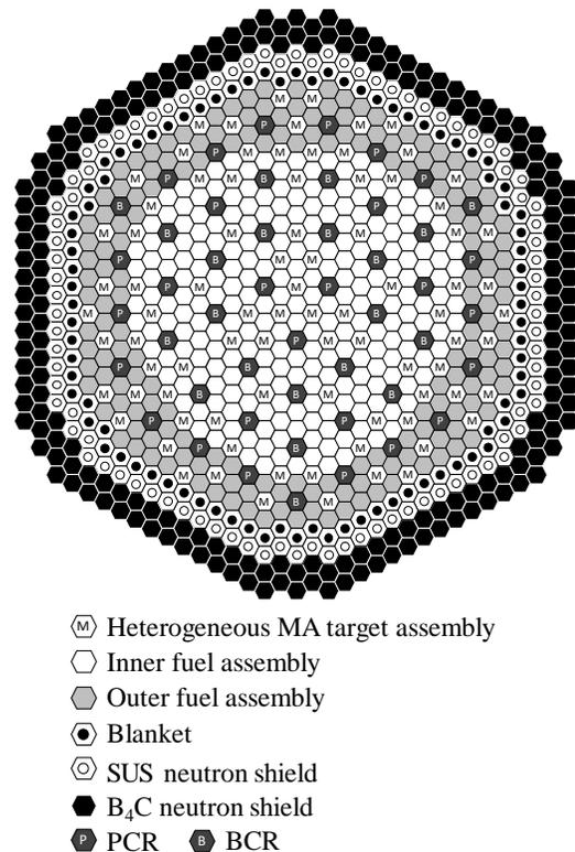
Fig. 1. Heterogeneous MA target loaded core
