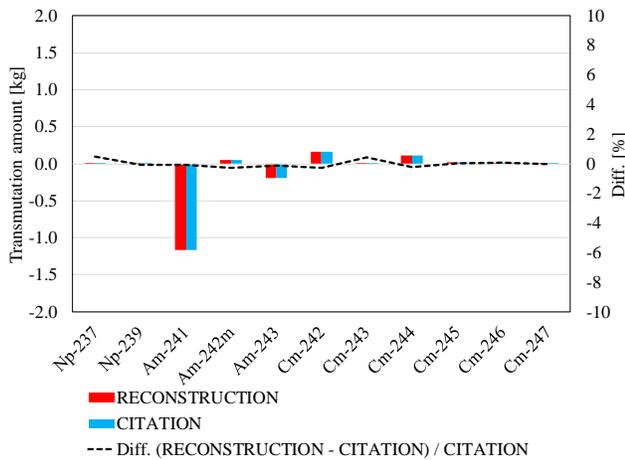
Fig. 13. Comparison of transmutation amount in assembly
