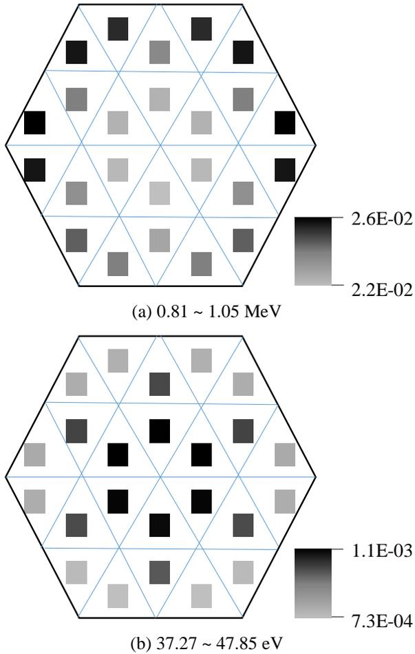
Fig. 3. Neutron flux distribution in MA target assembly
