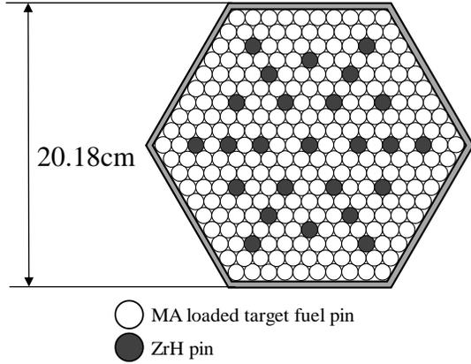
Fig. 2. Heterogeneous MA target assembly
