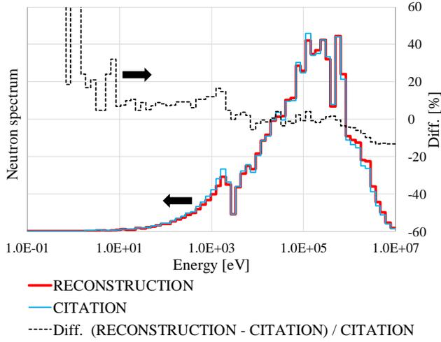
Fig. 7. Neutron spectrum in MA target fuel pin
