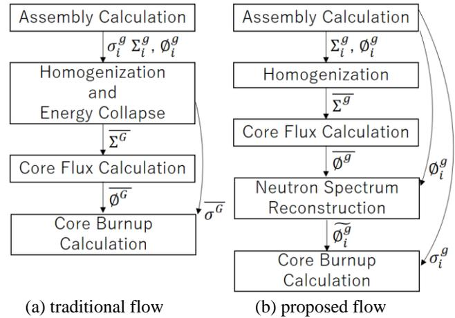
Fig. 4. Comparison of calculation flow
