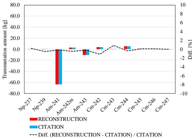
Fig. 14. Comparison of transmutation amount in all MA assembly
