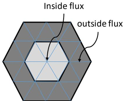
(b) inside flux and outside flux for quadric correction term
