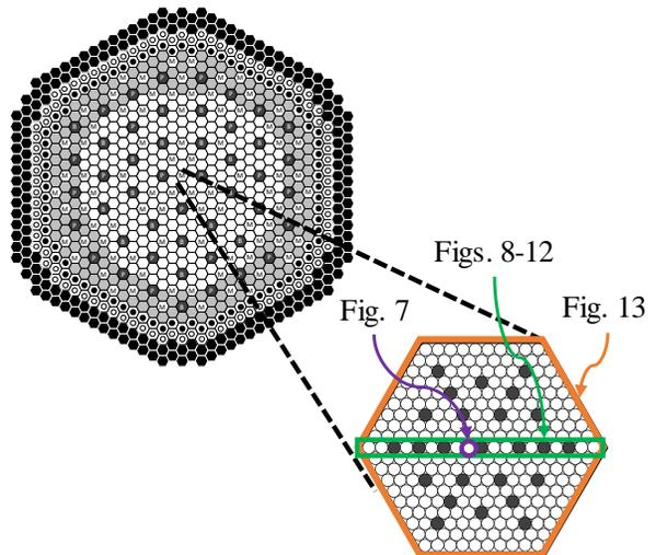
Fig. 6. Location of MA target assembly and pin
