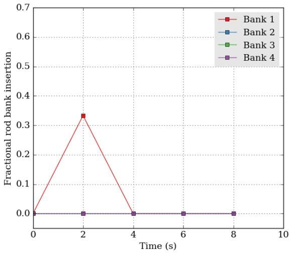
Fig. 6. Relative control rod position in exercise TD4-1.
