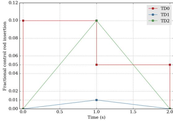
Fig. 4. Control rod movement in exercises TD0/1/2.
