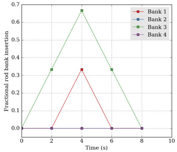
Fig. 8. Relative control rod position in exercise TD4-3.
