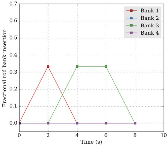
Fig. 10. Relative control rod position in exercise TD4-5.
