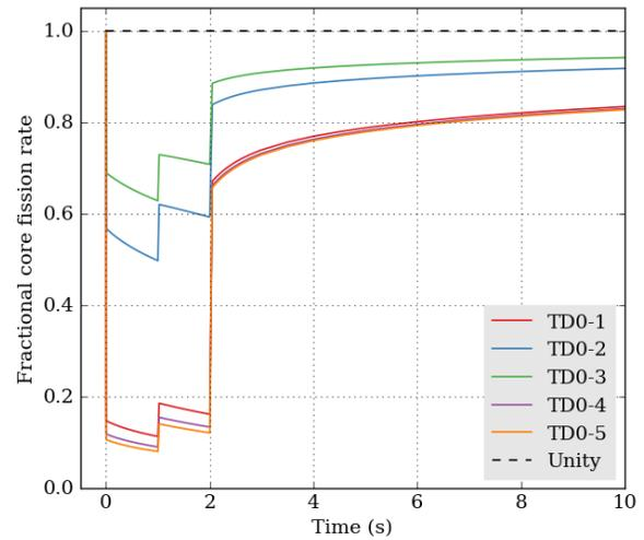
Fig. 15. Fractional core fission rate as a function of time for TD0 cases.
