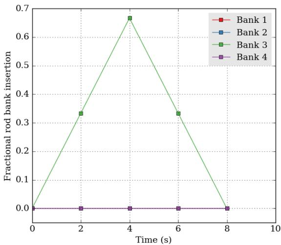
Fig. 7. Relative control rod position in exercise TD4-2.
