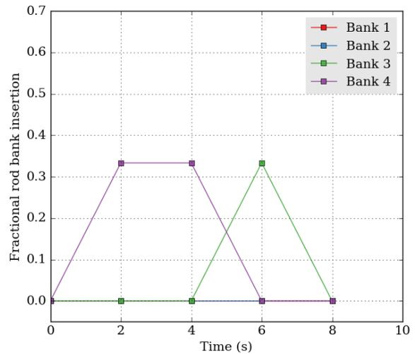
Fig. 9. Relative control rod position in exercise TD4-4.
