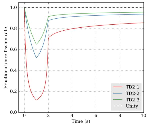
Fig. 16. Fractional core fission rate as a function of time for TD2 cases.
