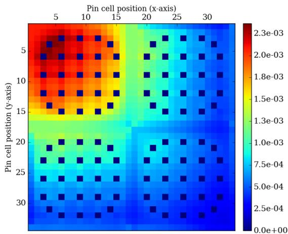
Fig. 14. Initial core fission rate distribution of C5G7-TD.
