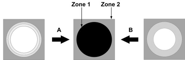
Fig. 3. C5G7 fuel pin compositions and numbering scheme.
