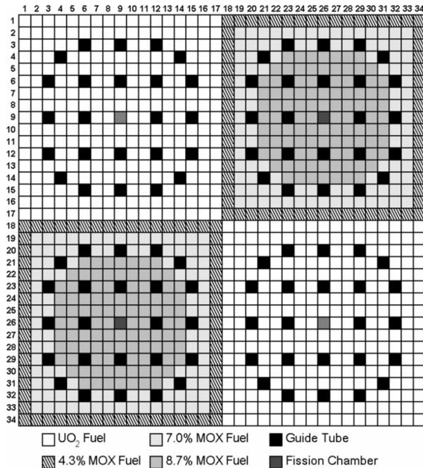
Fig. 2. C5G7 fuel pin compositions and numbering scheme.
