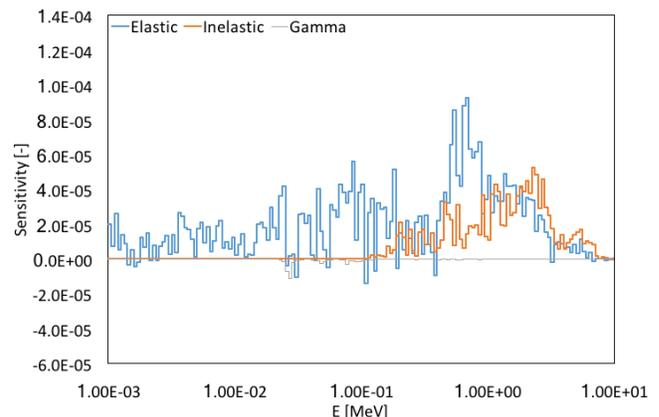
Fig. 8. Sensitivity profiles of scattering reactions on fluorine in FLIBE salt in fast energy region, compared with capture reaction.
