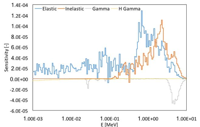
Fig. 7. Sensitivity profiles of scattering reactions on fluorine bound in Teflon in fast energy region, compared with capture reactions on fluorine and hydrogen.
