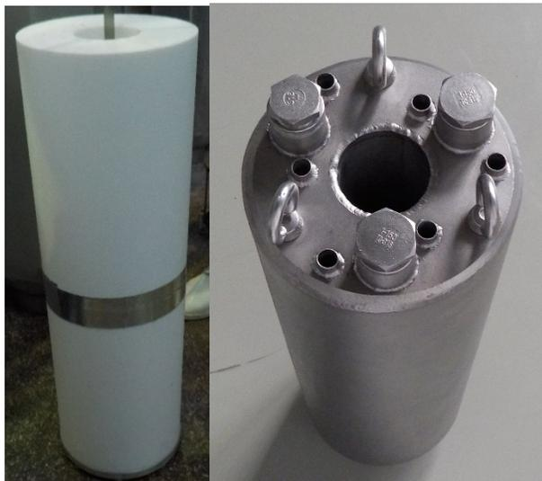
Fig. 3. Photographs of reactor insertions; Teflon cylinder (left) and canister with FLIBE salt (right).
