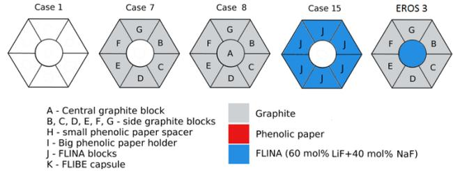
Fig. 4. Schematics of benchmark insertions. Cases 1, 7, 8, 15 and EROS3 are compared with recent results of Teflon and FLIBE.
