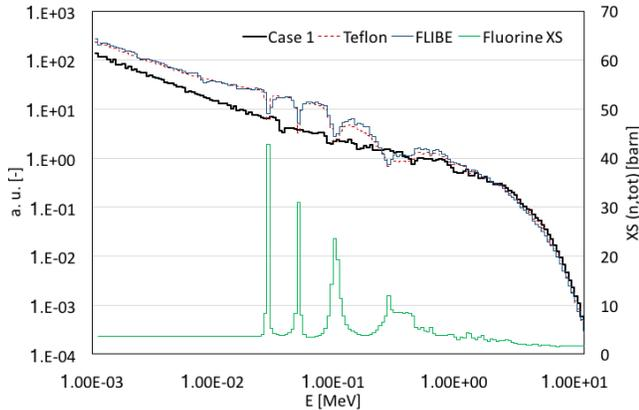
Fig. 6. Fast part of neutron spectrum calculated in Case 1 and experiments with Teflon and FLIBE.
