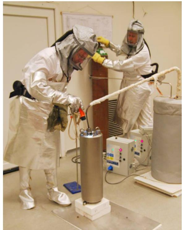
Fig. 2. Process of filling the FLIBE from transport cask into the canister used in irradiation channel of LR-0 reactor.
