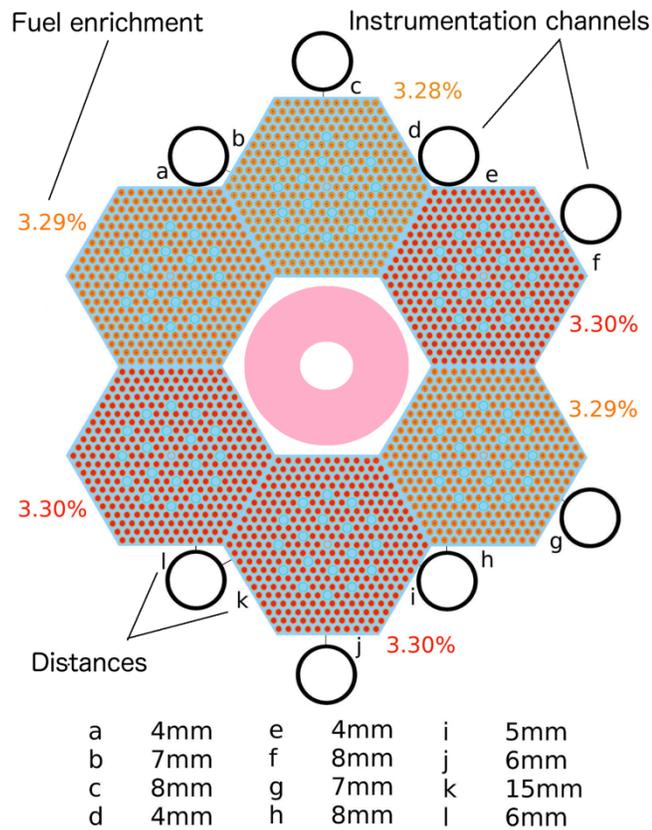
Fig. 1. Schematic view on the benchmark core in LR-0 reactor in configuration with Teflon insertion (in core center).
