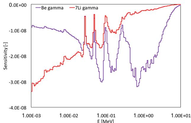
Fig. 9. Sensitivity profiles of radiative capture on Be and  ${}^7\text{Li}$  nuclei in FLIBE salt in fast energy region.
