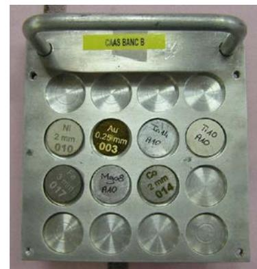
Fig. 4. Collimator Foil Holder with Neutron Activation Foils.
