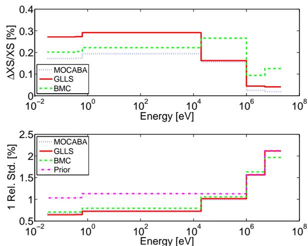
Fig. 3. Adjustments with each DA method to  $^{239}\text{Pu}/\bar{\nu}$  as  $\Delta\text{XS}/\text{XS}$  (above) and relative standard deviations (below).
