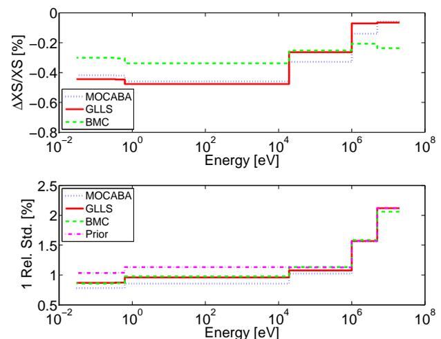
Fig. 6. Adjustments with each DA method to  $^{239}\text{Pu}/\bar{\nu}$  as  $\Delta\text{XS}/\text{XS}$  (above) and relative standard deviations (below).
