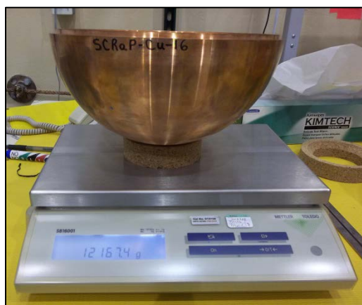
Fig. 3. A copper hemispherical shell for use in the SCRαP experiment.
