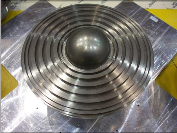
Fig. 1. 3.0 inch-thick Tungsten-Reflected Configuration with Top Reflectors Removed.
