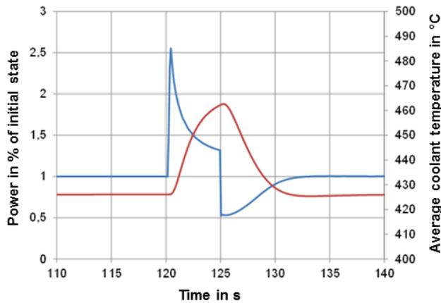
Fig. 15: Coupled PARCS/ATHLET simulation of a source transient in a MYRRHA core (preliminary). The blue line shows the power evolution, the red line the evolution of the average coolant temperature.
