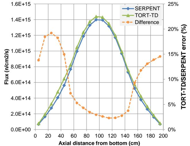
Fig. 6: Axial neutron flux profile of the TORT-TD diffusion solution compared with the Serpent reference simulation.
