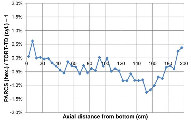
Fig. 9: Relative deviation of the hexagonal PARCS model axial flux distribution w.r.t. the cylindrical TORT-TD model.
