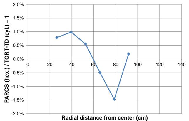
Fig. 10: Relative deviation of the hexagonal PARCS model radial power distribution w.r.t. the cylindrical TORT-TD model.
