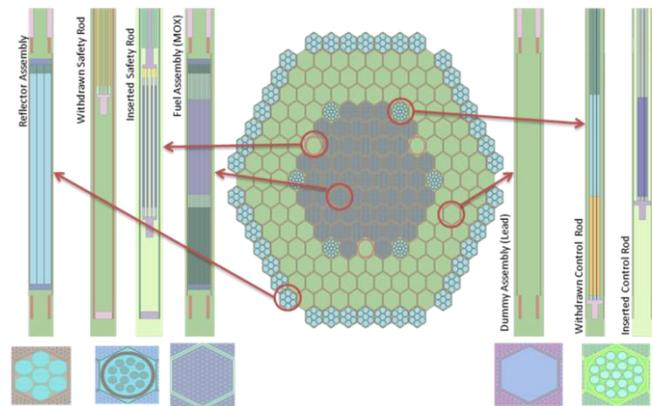
Fig. 14: Serpent model of the MYRRHA core (center) showing axial and radial subassemblies cross sections.
