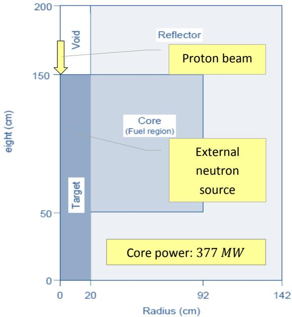
Fig. 1:  $r$ - $z$  model of the simplified accelerator-driven minor actinide burner system (modified from [8]).
