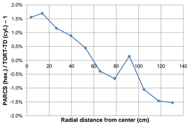
Fig. 8: Relative deviation of the hexagonal PARCS model radial flux distribution w.r.t. the cylindrical TORT-TD model.
