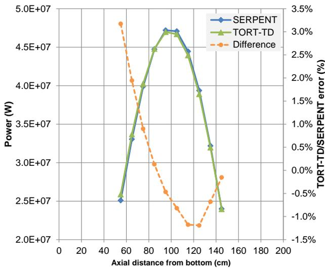
Fig. 4: Axial power profile of the TORT-TD diffusion solution compared with the Serpent reference simulation.
