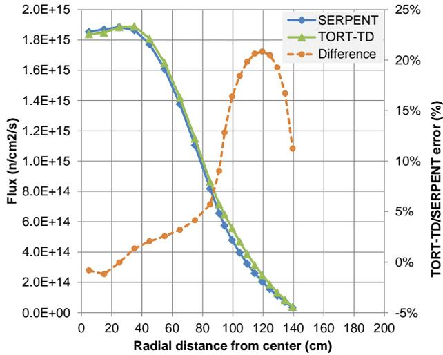
Fig. 7: Radial neutron flux profile of the TORT-TD diffusion solution compared with the Serpent reference simulation.
