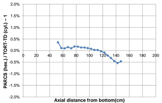
Fig. 11: Relative deviation of the hexagonal PARCS model axial power distribution w.r.t. the cylindrical TORT-TD model.
