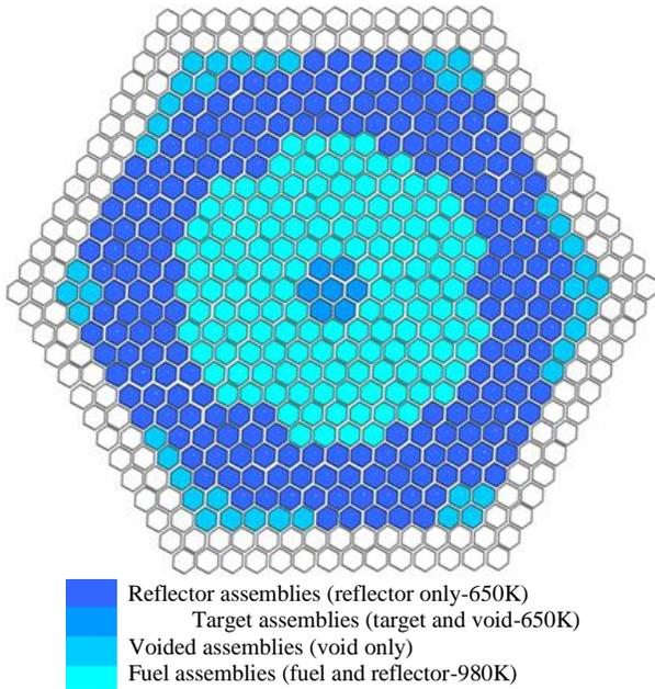
Fig. 2: Hexagonal radial core configuration equivalent to the cylindrical core.
