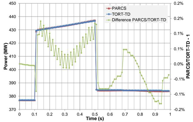
Fig. 13: Total power evolutions during the source transient obtained with PARCS (green line) and TORT-TD (blue line). The purple line denotes the relative difference between both codes.
