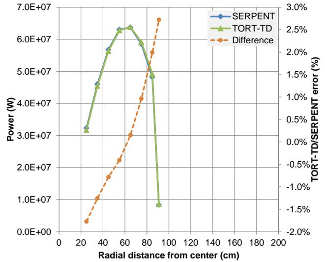
Fig. 5: Radial power profile of the TORT-TD diffusion solution compared with the Serpent reference simulation.
